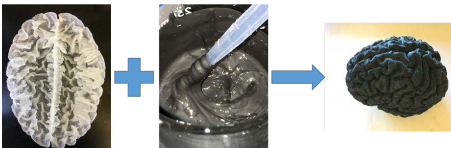
Figure 1. Constructing the brain phantom by the shell method where the conductive polymer is casted into the brain shell.
