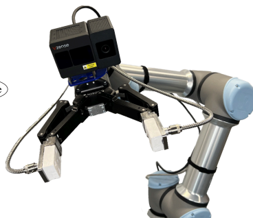
Figure 1. Robotic magnetic gripper design and effector combined with robotic base.
