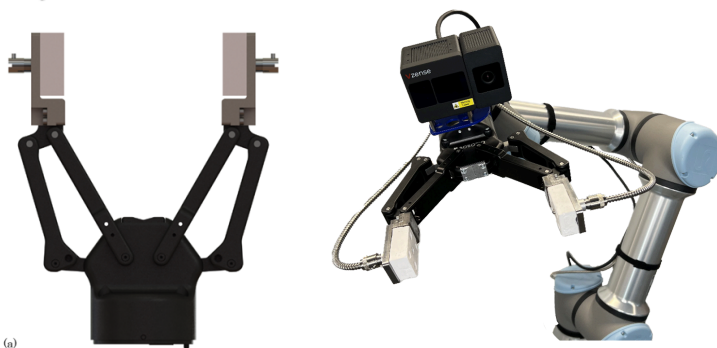
Figure 1. Gripper arm 3D diagram and robotic gripper fitted with a camera for remote control.
